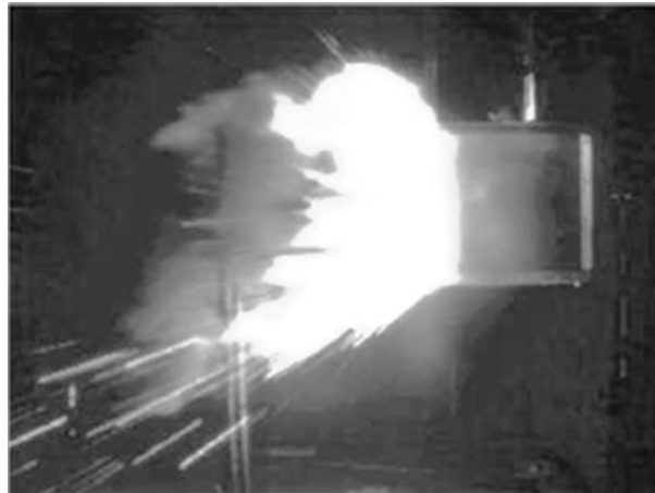
Figure 1.2: Simulated arc-flash incident, conducted at 250V, 13.1 KA (13,100 amps). Energy intensity: 1.48 Cal/cm 2 .
